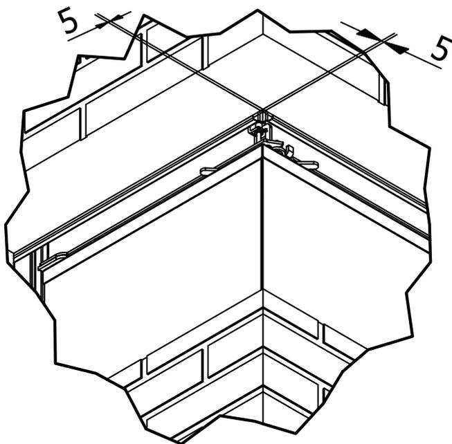
Due to the stoves structure there will be air gaps of 34 mm to the sides and the bottom, which can be closed e.g. with non-combustible panels.
