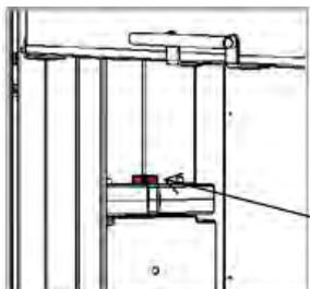
**4. Tighten the retaining ring (Allen key 2.5mm).**
