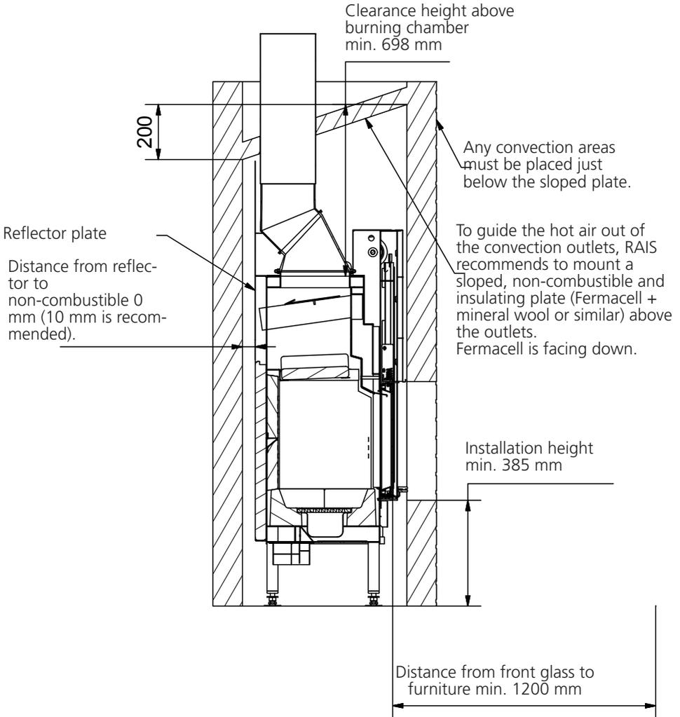
Construction of sloped plate.
