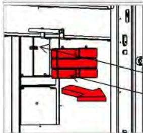
**3. Unscrew the retaining ring (Allen key 2.5mm). Remove the required number of counterweights, so that the door closes slowly and at a constant speed. Check its operation.**
