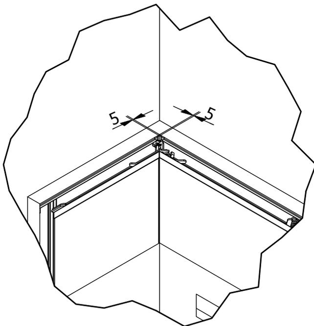
Due to the stoves structure there will be air gaps of 34 mm to the sides and the bottom, which can be closed e.g. with non-combustible panels.
