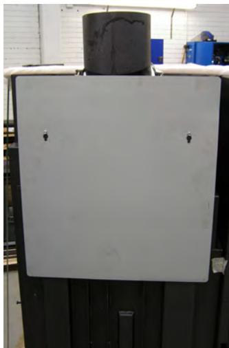
Dismount the reflector plate and turn it upside down. Mount the plate reusing the screws (as shown).
