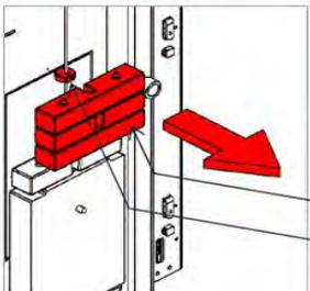
**3. Remove the retaining ring (Allen key 2.5mm). Remove the required number of counterweights, so that the door closes slowly and at a constant speed. Check its operation.**
