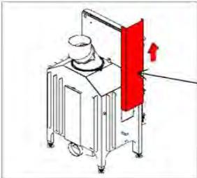
**2. Remove the counterweight cover by pulling it up.**
