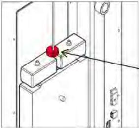
**4. Tighten the retaining ring (Allen key 2.5mm).**
