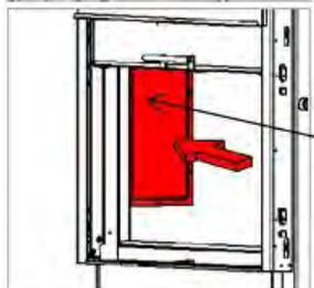
**5. Refit the access panel and side Skamol sheet.**
