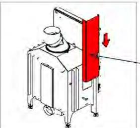
**5. Attach the counterweight cover and screw in the screw(s).**
